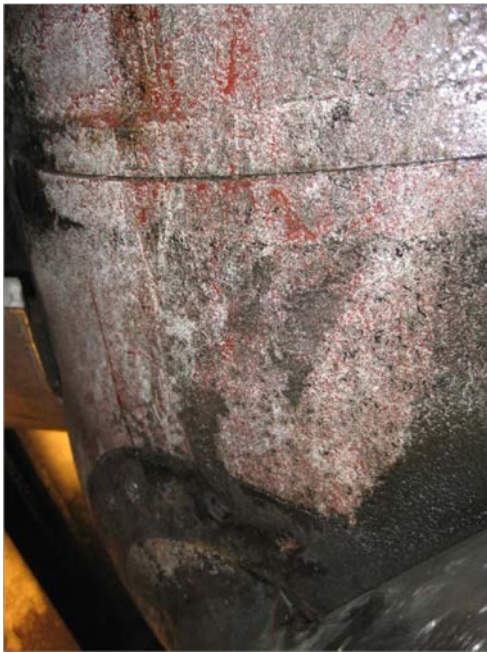
Figure 7. Stainless Steel Overlay on the Blades Suction Side (Underside, Leading Edge)
