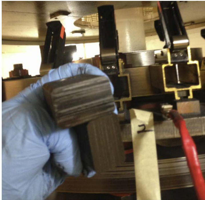
Photo 1: Brush threading and uneven wear
