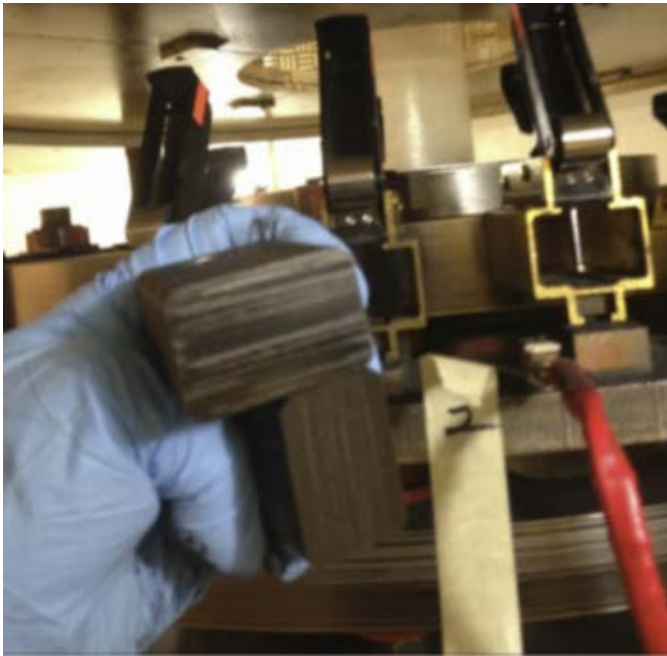
Photo H. Brush Threading and Uneven Wear
