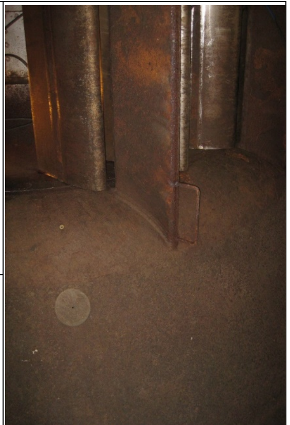
Figure 11. Discharge Ring SS Repair Shown below a Blade with a Cavitation Fin
