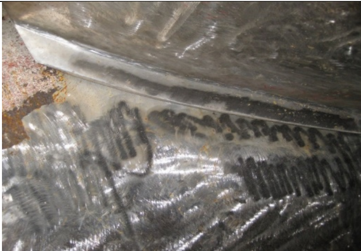
Figure 12. Add'l Photo Showing Wicket Gates & Stay Vane with a Corrosion Patina
