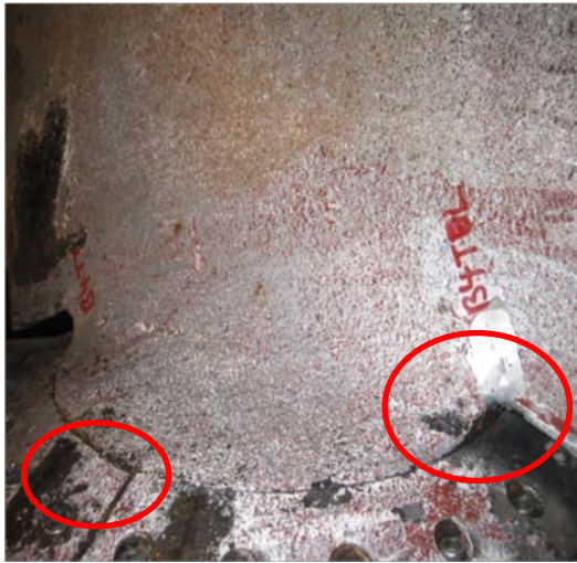
Figure 9. Blade Cracks That Have Been Repaired and Are Not Re-Cracking
